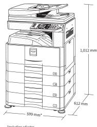
\*Including adjuster. 909 mm when multi-bypass tray is extended.
